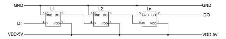
Depending on the power supply quality, a filter capacitor can be appropriately added in parallel between GND and VDD (it is recommended to take a value of 100nf).
