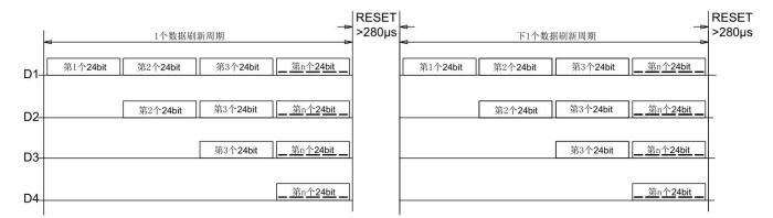
Note: Among them, D1 is the data sent by the MCU end, and D2, D3, and D4 are the data automatically shaped and forwarded by the cascaded circuit.
